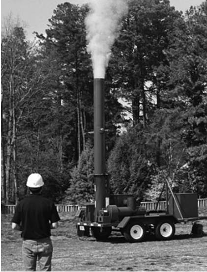
Learning to read smoke opacity on a smoke machine during "Smoke School"
