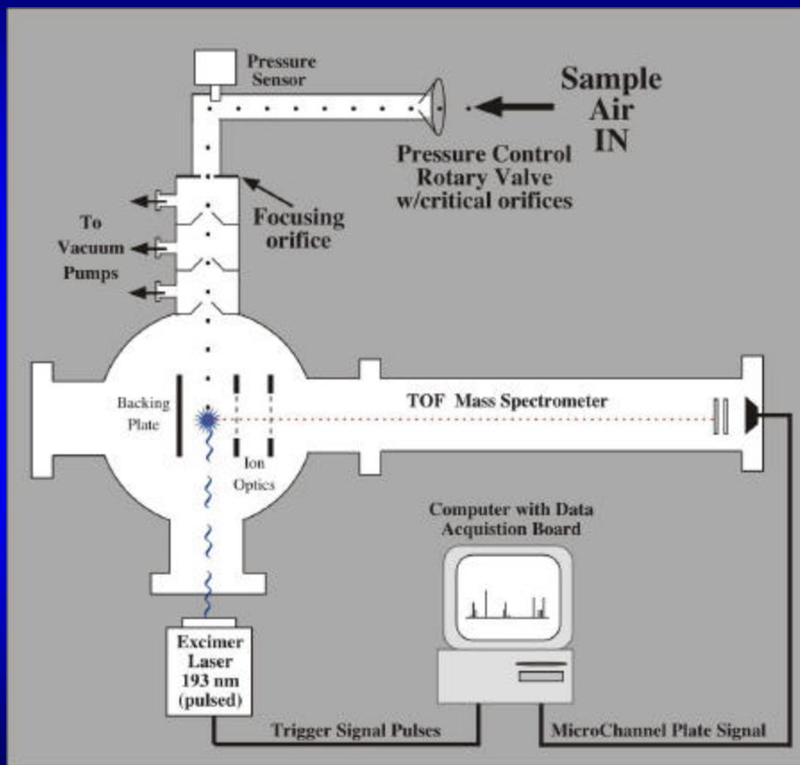
**RSMS – Single Particle Mass Spectrometer**
