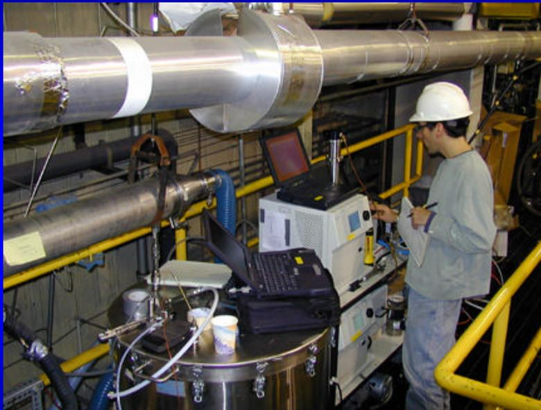
Dilution sampling on a pilot-scale combustor
