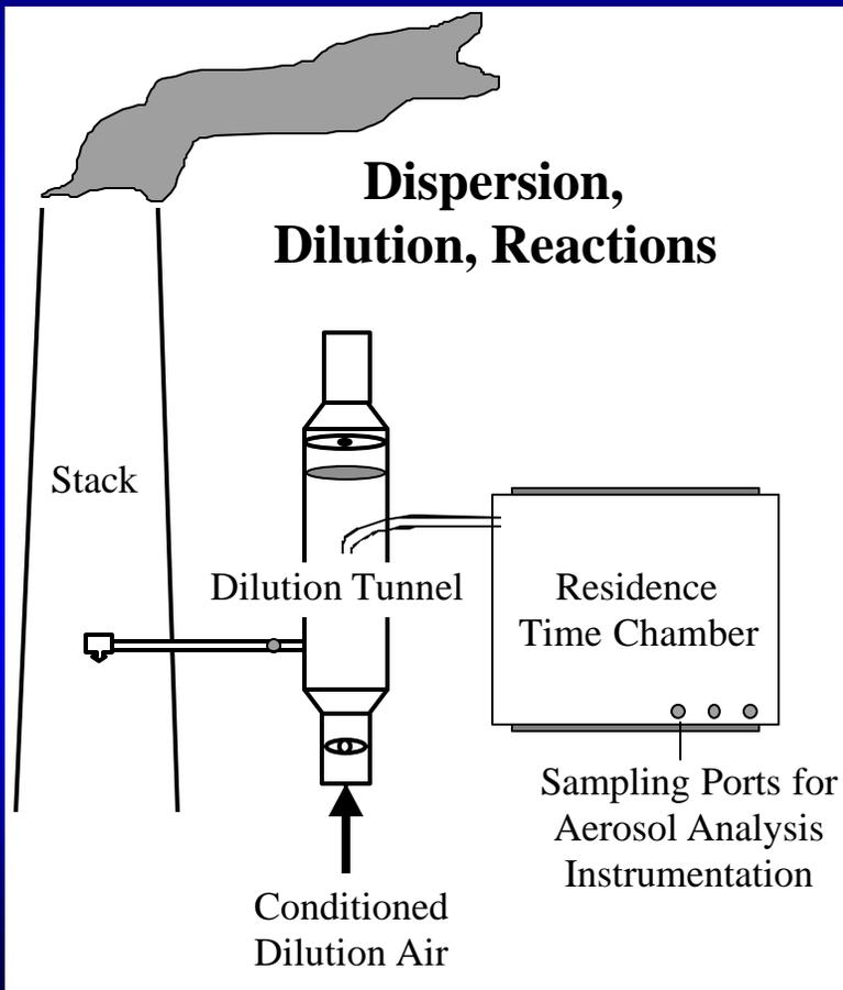
Schematic of Portable Dilution Sampler
